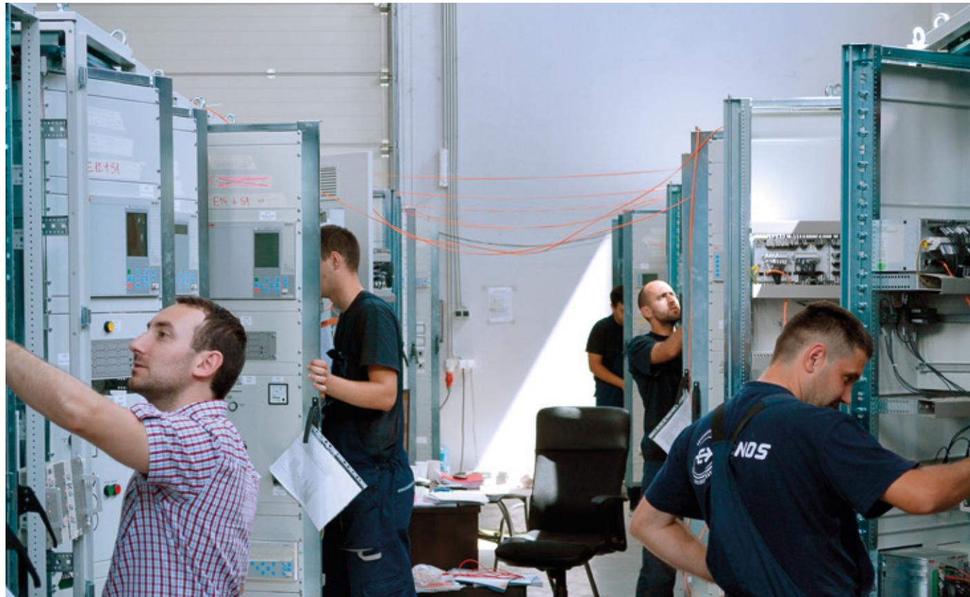
Montaža ormara reljejne zaštite i upravljanja / Installation of relay protection and managing cabinets
